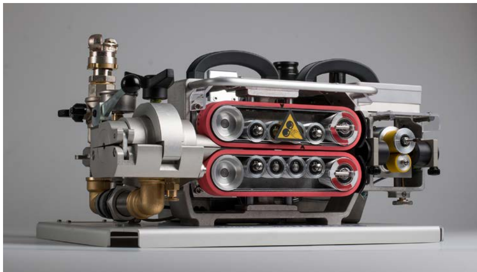
The red drive belts push the cables into the tubes. The new coating allows an optimal cable grip.
